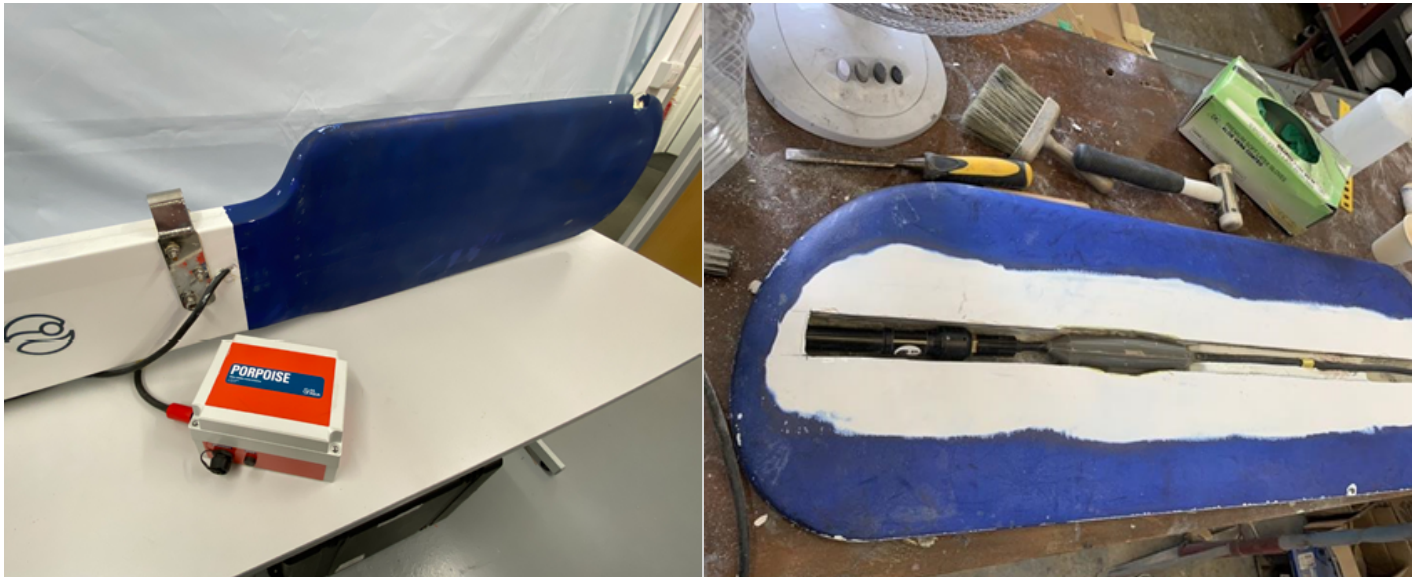
Image of the RS Aqua Porpoise hydrophone integrated with the rudder of a GB Row Challenge boat.
